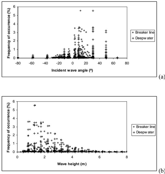
Figure 2. Frequency of occurrence of the (a) incident wave angles and (b) wave heights of the complete wave regime.
